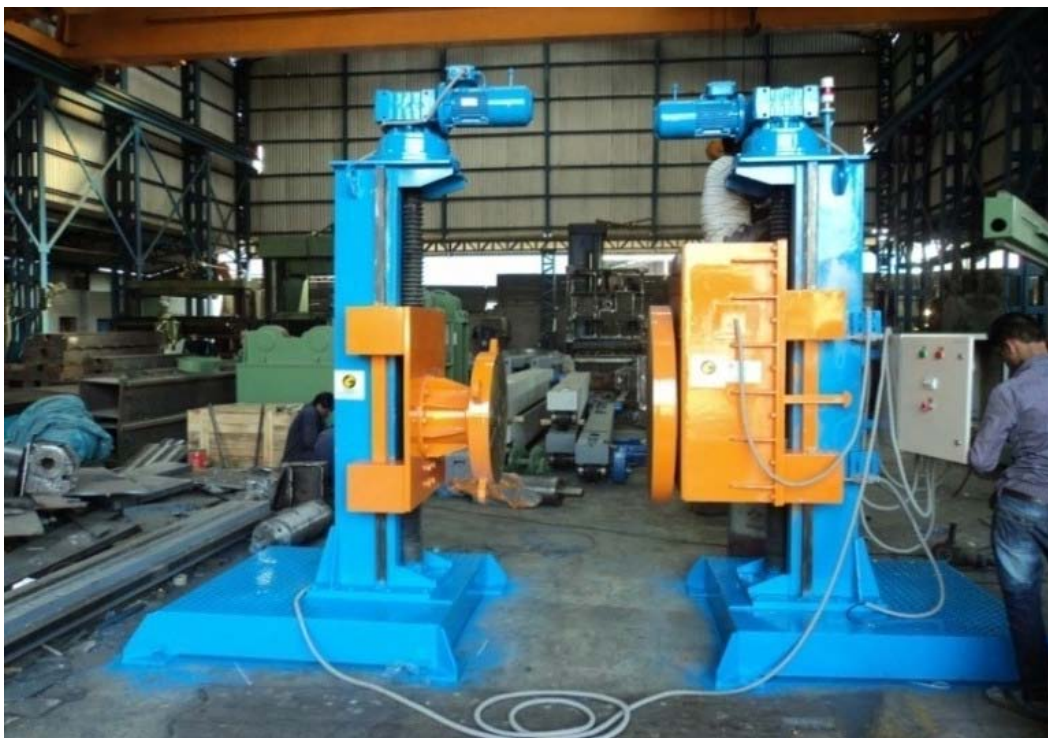
2 Axis HSTS Manipulator supplied to Indian Coach Factory through Kuka Systems for Bogie Frame
