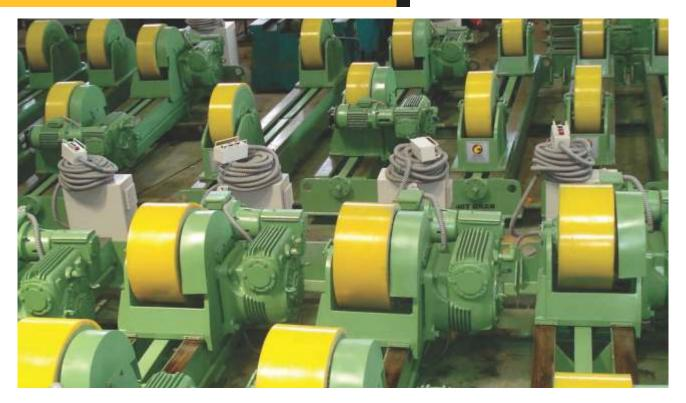
Welding Rotators are very essential equipments for heavy and light fabrication shop. They are mainly used to rotate or position the cylindrical jobs for circumferential welding (TIG / MIG / Sub Arc) or for intricate assemblies. The machine consists of 1 No. Drive Unit and 1 No. Idler Unit and Control panel with pendant. For step less speed variation, AC Variable Frequency Drive is used. The rollers are either made of Steel or Moulded with Polyurethane as per customer's requirement.
