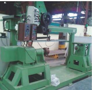
We design and manufacture any Special Purpose machine for Automatic/ Semi-automatic/Manual Welding. These SPMs may use any welding process as required for the specific job. The welding process may be MIG / MAG, TIG, or SAW. Some of the SPMs we have manufactured for various customers are as follows:
